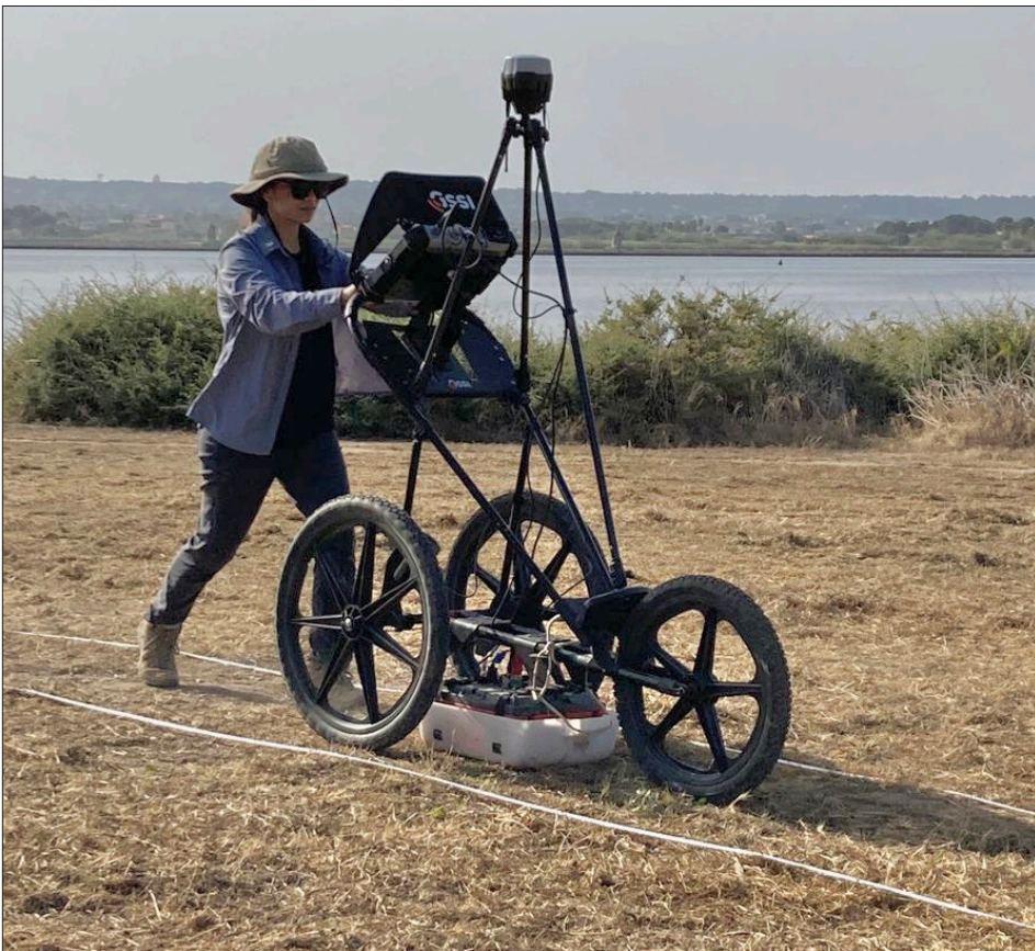
Figure 44: Helen Wong (AAMW) conducting ground-penetrating radar (GPR) survey at Mozia, Sicily.
